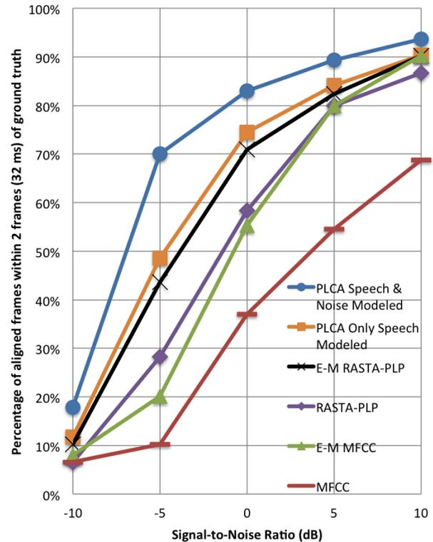
Fig. 3. Percentage of aligned frames within 2 frames (32 ms  $\approx$  1 video frame) of correct alignment
