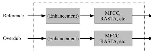
(b) Block diagram of conventional feature extraction method
