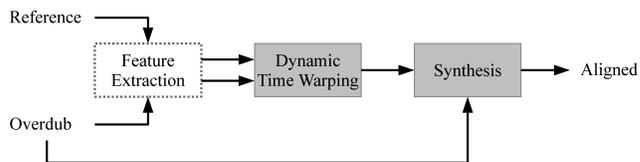
(a) Block Diagram of three-stage automatic alignment system
